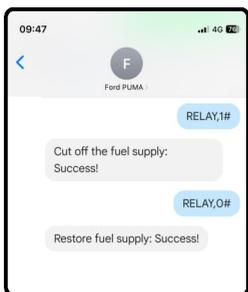
**Once the command is sent, (via APP or SMS) the relay will be activated only if the speed is less than 20 km/h preventing the vehicle from starting.**
